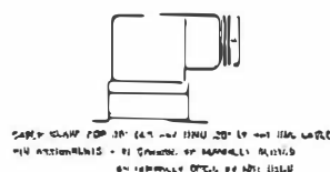
COMPLETE DIN - OPTION "HR" • DIN 43650-A TYPE • PLUG AND RECEPTACLE INCLUDED
